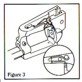
of the barrel. The base pin must be fully inserted and locked in position by the base pin latch. If the base pin is not fully inserted and locked, the transfer bar may catch under the firing pin when the hammer is being cocked.
