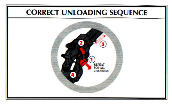
Do not eject unfired cartridges onto any surface where the cartridge primer might strike a solid object and discharge the cartridge.
