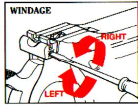
To move the point of impact to the <u>right</u>: turn screw counterclockwise.
